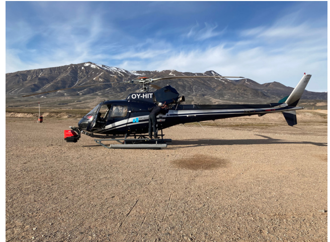
Helicopter equipped for hyperspectral data acquisition. Kap Simpson, NE Greenland, Ministry of Mineral Resources and Justice. 2022
